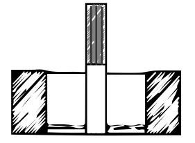
STEP 3 Insert provided PVC Adapter over the Rebar. Once Inserted fill the rest of the PVC with concrete including the new Adapter.
